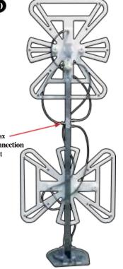
Thread the existing coax cable between the boom and the center of the upper element housing.
