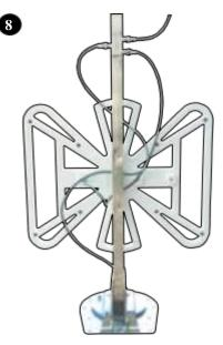
Connect the coax to the coax connection port, and tighten until fingertight. Then, tighten <sup>1</sup>/<sub>4</sub> turn more.
