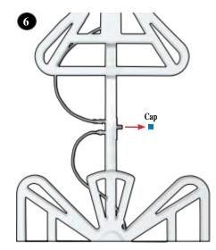
Remove the cap from the coax connection port.
