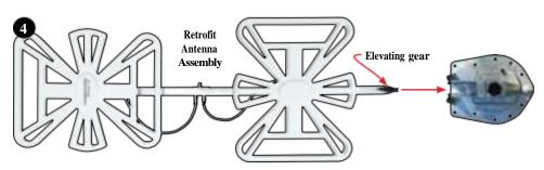
Using the retrofit antenna assembly, insert the elevating gear in-between the sides of the leveling bracket. The elements should be on top of the boom. The holes in the sides of the leveling bracket and in the elevating gear should align.
