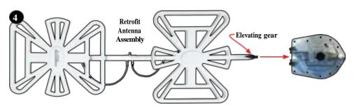
Using the retrofit antenna assembly, insert the elevating gear in-between the sides of the leveling bracket. The elements should be on top of the boom. The holes in the sides of the leveling bracket and in the elevating gear should align.
