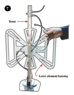
Thread the 140 cm coax between the boom and the center of the lower element housing. Continue to thread the coax in an S-curve between the boom and the center of the lower element housing.
